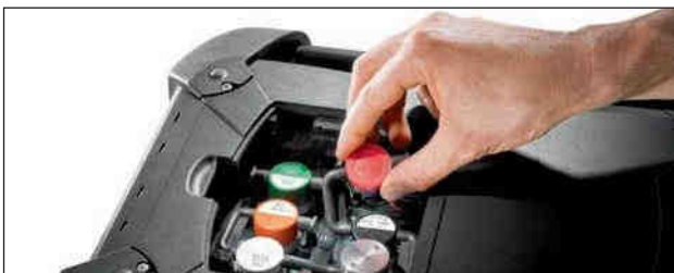
Plug & play: Easy gas sensor replacement
