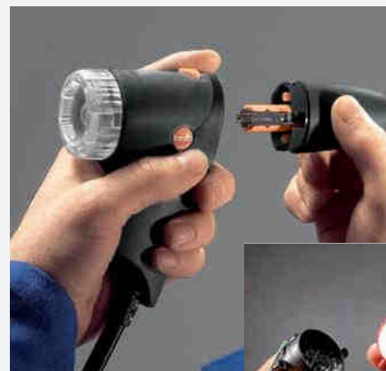
Exchanging probe shaft
